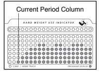
ting for the first period will be shown in the flashing Current Period column of the program display. (The incline settings are not shown in the program display.) The speed settings for the next seventeen periods will be shown in the seventeen columns to the right.
